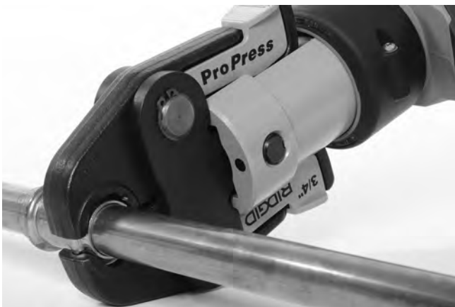
Figure 9 – Placing Scissor-Style Jaws Around Fitting
