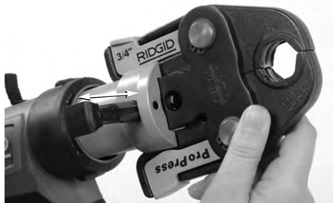
Figure 7 – Attachment Mounting Pin
