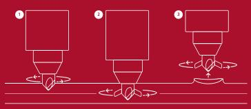
1. Drilling of pilot hole 2. Extension of forming pins 3. Finished collar
